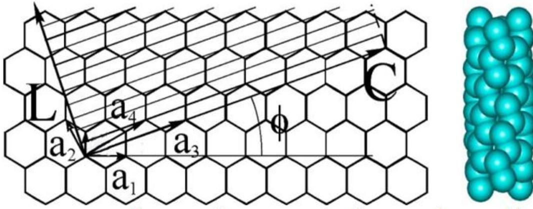
Fig. 1. A graphite layer and carbon tube with chirality indices (9,3) basis vectors  $(\mathbf{a}_1, \mathbf{a}_2)$ ,  $(\mathbf{a}_3, \mathbf{a}_4)$ , chirality angle  $\varphi$ .
