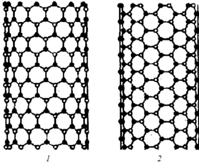
Fig. 3. Zigzag - 1 and armchair - 2 tubes of boron nitride.
